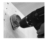
**10.** Push rod against wall in "non-wired" flange and tighten set screw.
