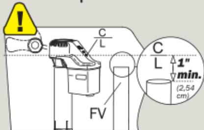
c) Attach tube to flush valve (FV) with metal clip so water flows into flush valve. Trim tube if kink occurs.
