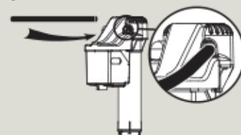
Tip: Run tube under warm water for easier install.
