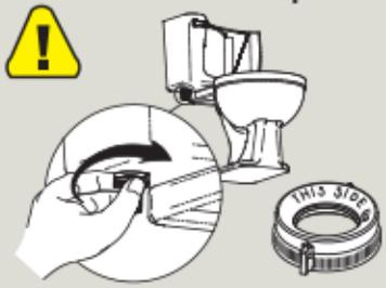
b) **Confirm critical level (C/L)** is 1" above flush valve (FV).
